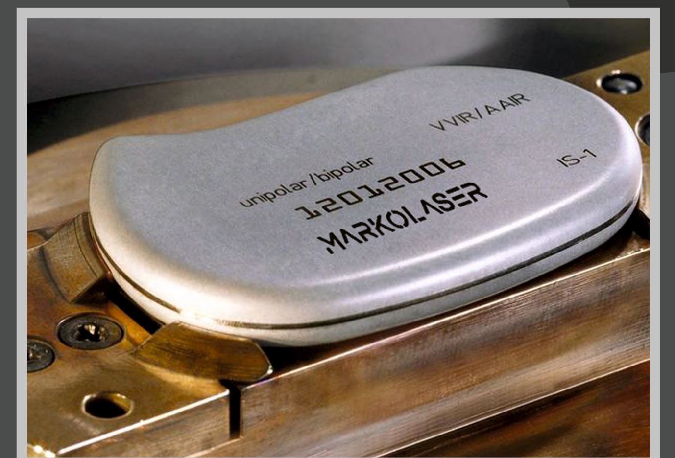
Heat Conduction Welding on Medical Implants
