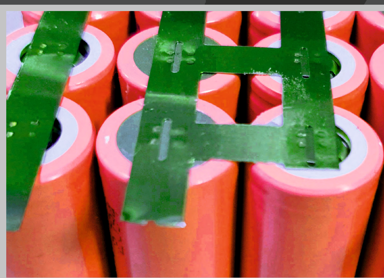
Laser Spot Welding on Li-ion Battery Tab
